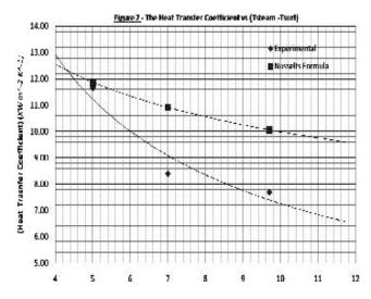
condenser (3). As a relatively poor conductor of heat, this film creates a thermal resistance which is the reason why the value for Heat Flux is lower for filmwise in comparison to dropwise condensation (3)
