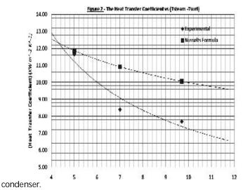
The vapour drops in dropwise condensation are discrete and are continually formed and released which means that the surface of the condenser is alsocontinually exposed. In comparison, the film created in filmwise condensation always covers the surface of the
